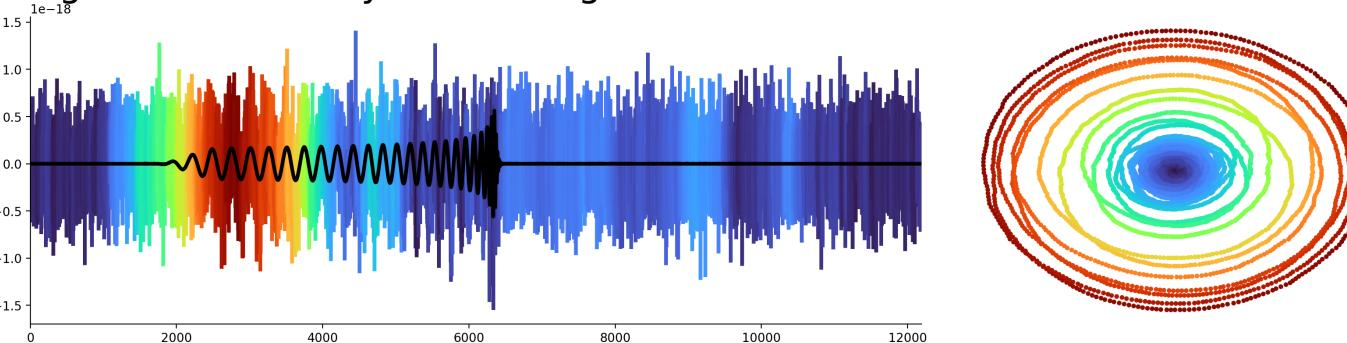
The hidden signal (black) in the noise is revealed through the time delay embedding. Window Size = 70
